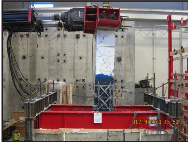
Figure 2. Testing of Repaired Column
